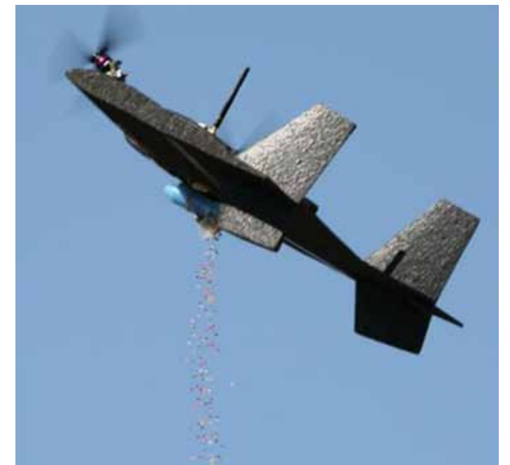
The Skate small UAS performs a taggant payload dispersal test in flight during a series of experiments conducted at Camp Roberts, Calif. The project is part of Marine Corps Capt. Dino Cooper’s thesis project on UAS taggant delivery.
