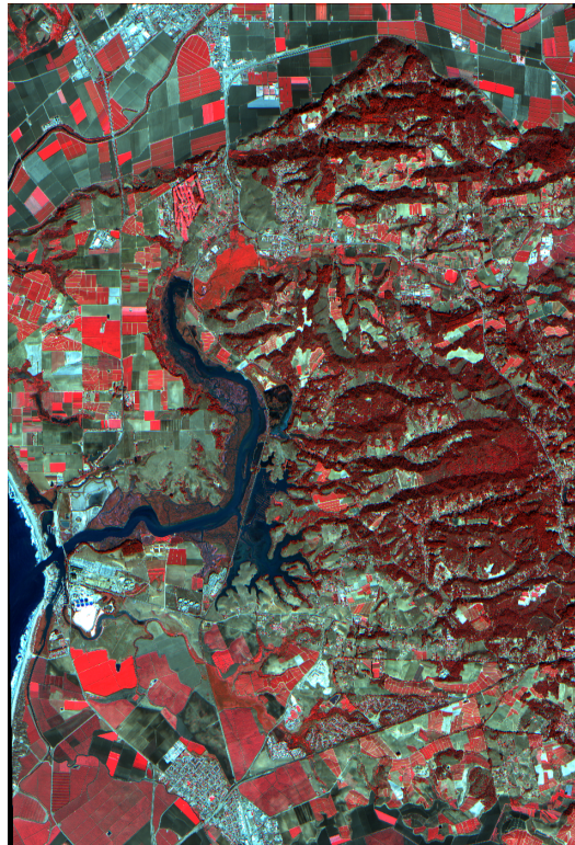
Figure 1. IKONOS image of Elkhorn Slough, October 23, 2000. Bands 4 (NIR), 3 (red), and 2 (green) are presented as a false-color infrared image. The image is 10 km x 20 km. North is to the top.
