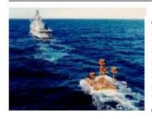
The Test Ship tows a Decoy Barge 100 yards astern. The barge seduces inbound cruise missiles away from the ship to prevent damage to the test ship and its combat systems payload.
